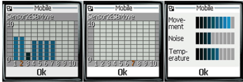
Figure 9.14.: The visualization of the given sensor values. 1. and 2. The simple sensor request, 3. Get awareness.
